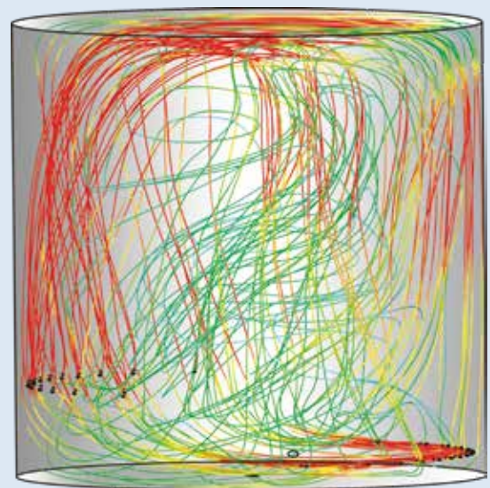
Optimisation of the flow conditions in a cylindrical storage tank for edible oil through three dimensional computer simulation. Vertical section; spatial distribution of the flow velocity as a coloured halftone image
